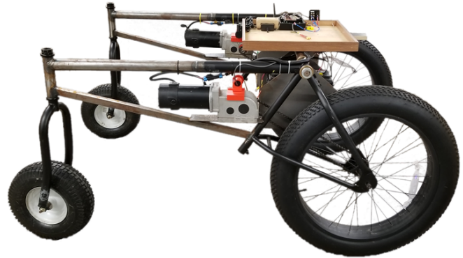
Fig. 1: Rx Robotics autonomous horticultural rover, the ‘bikebot’. The rover is currently an electrical powered wheeled vehicle, which will be remodeled with tracks.
